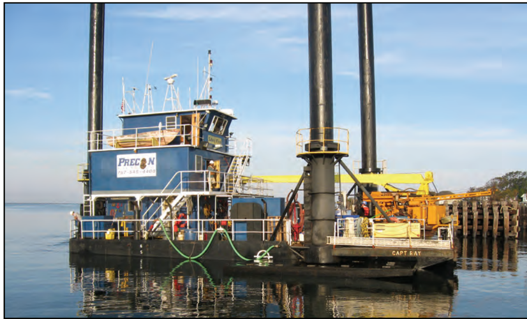
Jack-Up Barge – Deep Geotechnical Investigation Platform
