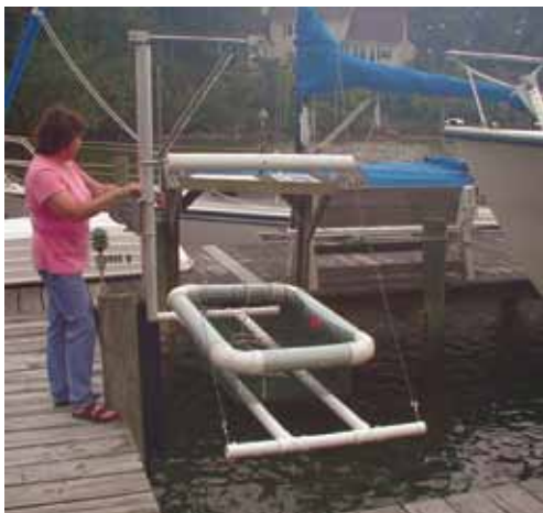
Gardeners have devised ways of lifting floats up to the dock for cleaning and maintenance. Small cranes, boat lifts, even jet-ski lifts may be adapted for this purpose. Photo courtesy of TOGA.
