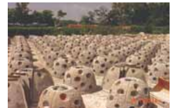
Reef Balls manufactured for artificial fishing reef deployment.
