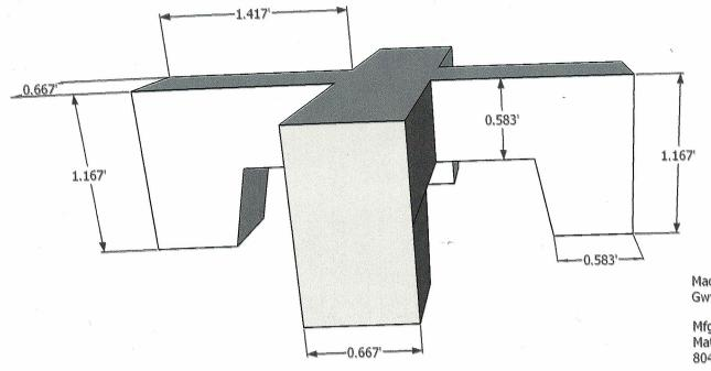
42" W x 14" H X-Reef @ 250 lbs Oyster Shell Veneer; Crack Resistant concrete substrate with rebar reinforcement
